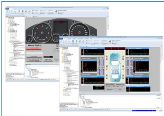
ControlDesk from dSPACE lets users define controls, knobs, dials, and gauges to connect to parameters within the model.
