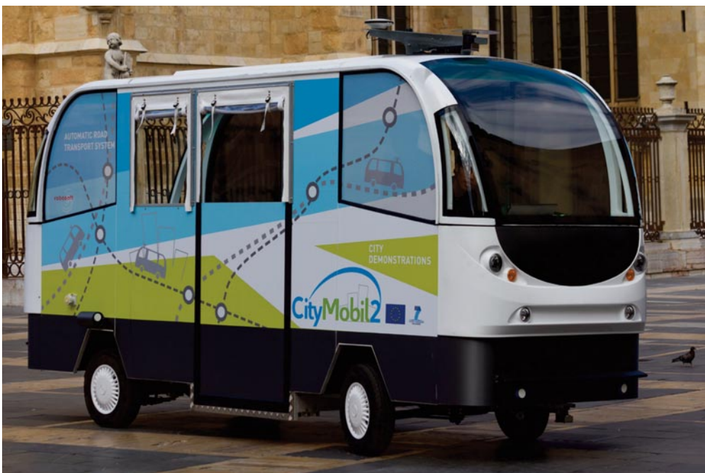
Prototype tests of a driverless minibus have been conducted in Spain. The CityMobil 2 electric bus can carry up to 10 passengers and reach a top speed of 40 Km per hour.
